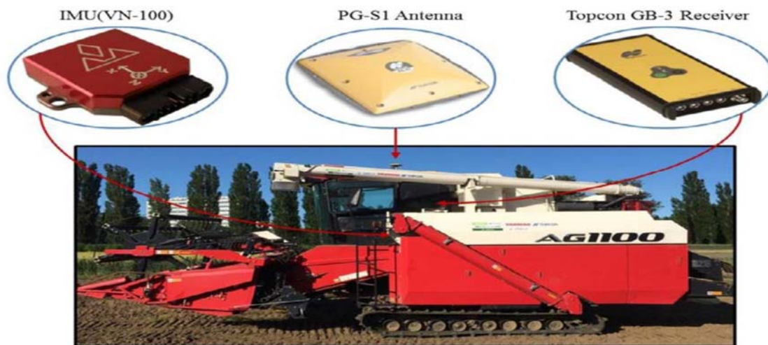
Figure 1: Outlook of the tracked combine harvester equipped with RTK-GPS and IMU sensors.
