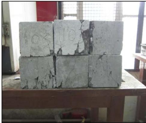
Fig.3: Typical Mode of Failure for Cubical Specimens.
