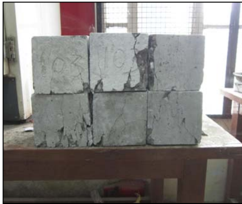
Fig.3: Typical Mode of Failure for Cubical Specimens.
