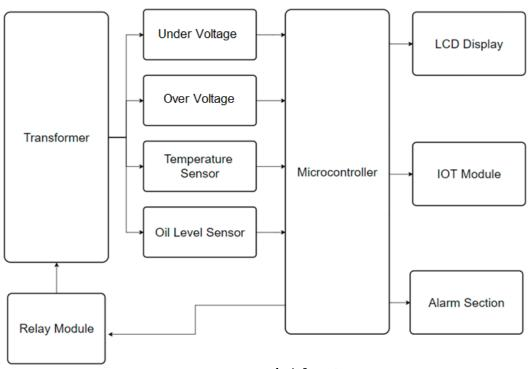
Description: Transformer is a static device which convert the voltage from one level to other level without change in frequency and power. Load is connected at secondary winding of the transformer. Due to many factor suddenly increase in load can cause overloading, overvoltages and overheating that can harmful to the transformer windings insulation and severe damage can be occur on the secondary side of transformer.
