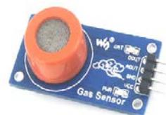
Gas sensor is one which comes handy in applications where we have to detect the variation in the concentration of toxic gases in order to maintain the system safe and avoid/caution any unexpected threats.
