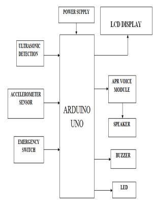
1.An ultrasonic sensor detects the obstructions using sound waves. It emits a sound wave of a certain frequency and waits for it to return. The elapsed time between these two events can be used to calculate distance. An ultrasonic sensor is used in the suggested device, which has a theoretical measurement distance of up to 3m.
