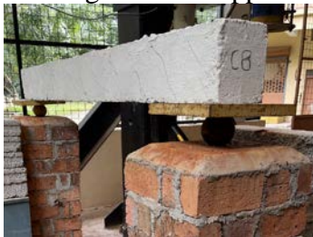
Fig.4: Specimen placed on supports
