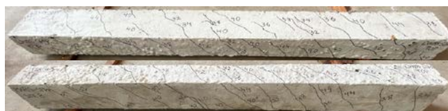
Fig 14. Continuous spiral cracks of hybrid fibre reinforced light weight beam with silica fume
