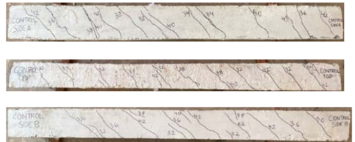
Fig 9. Crack patterns on the sides and top face of control beam
