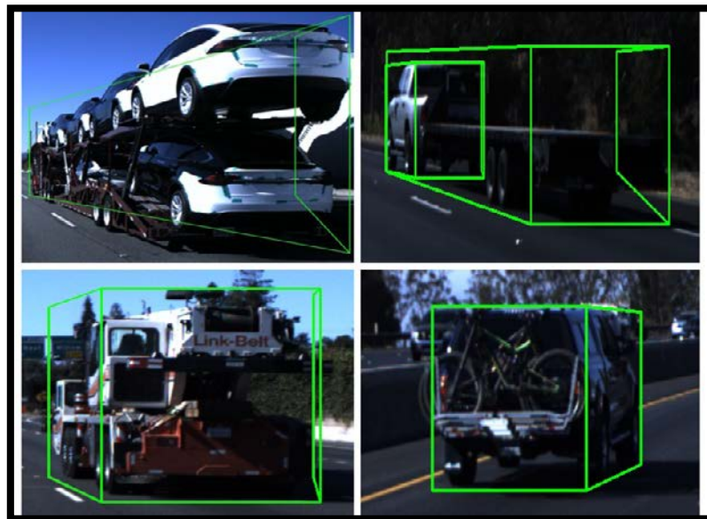
Fig 1.2 Example of vehicle detection using bounding boxes
