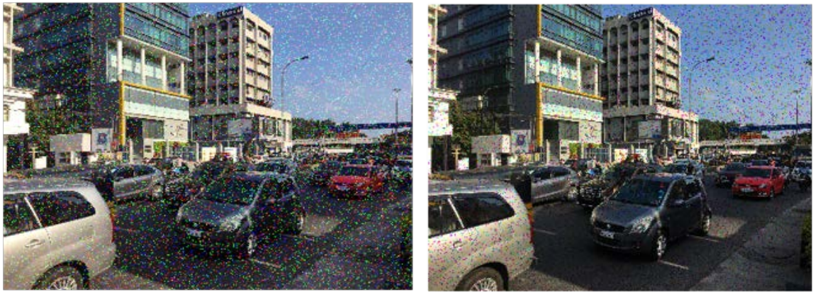
Fig 8.7 Image after applying (a) Salt and (b) Pepper Noise
