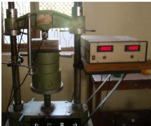
Figure 7: Plywood in Compression Testing Machine
