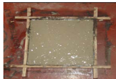
Figure 5: Casting in tile mould
