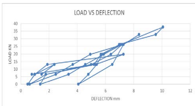
CYCLIC LOAD FOR WELDED MESH SLAB
