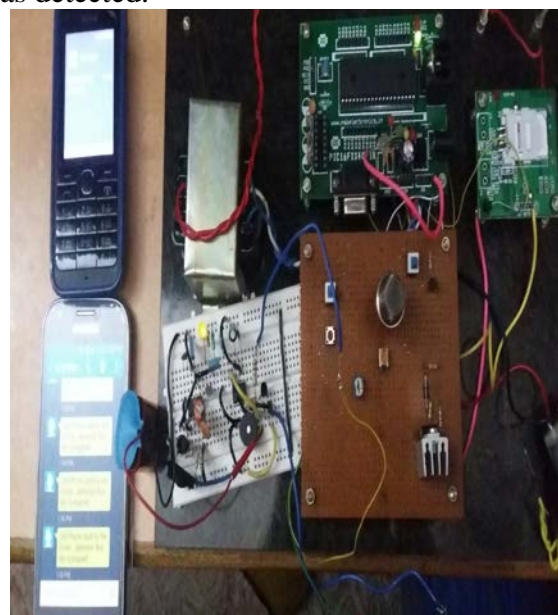
Figure 7.4 Call detector output – Reporting unit
