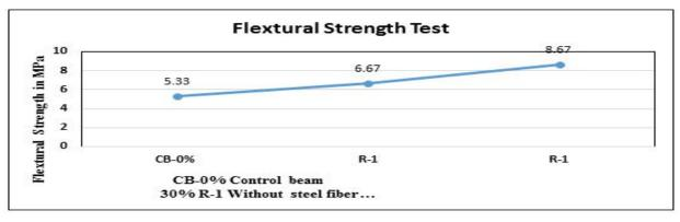
Fig 2: Flexural strength test results
