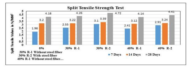
Fig 2: Split tensile Strength test
