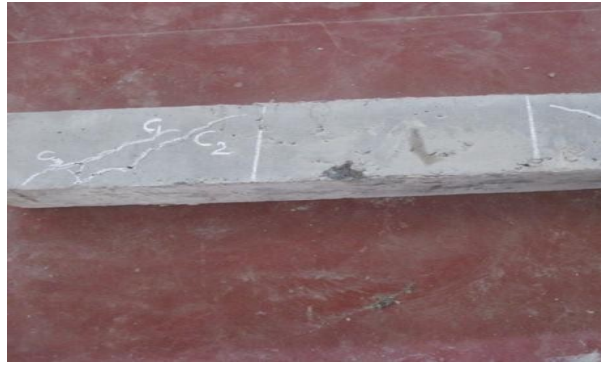
Fig 6 Cracks on control specimen
