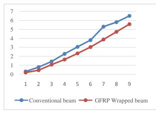
6.1.5 FLEXURAL STRENGTH OF RC BEAM (L/3 span) DEFLECTION OF RC BEAM
