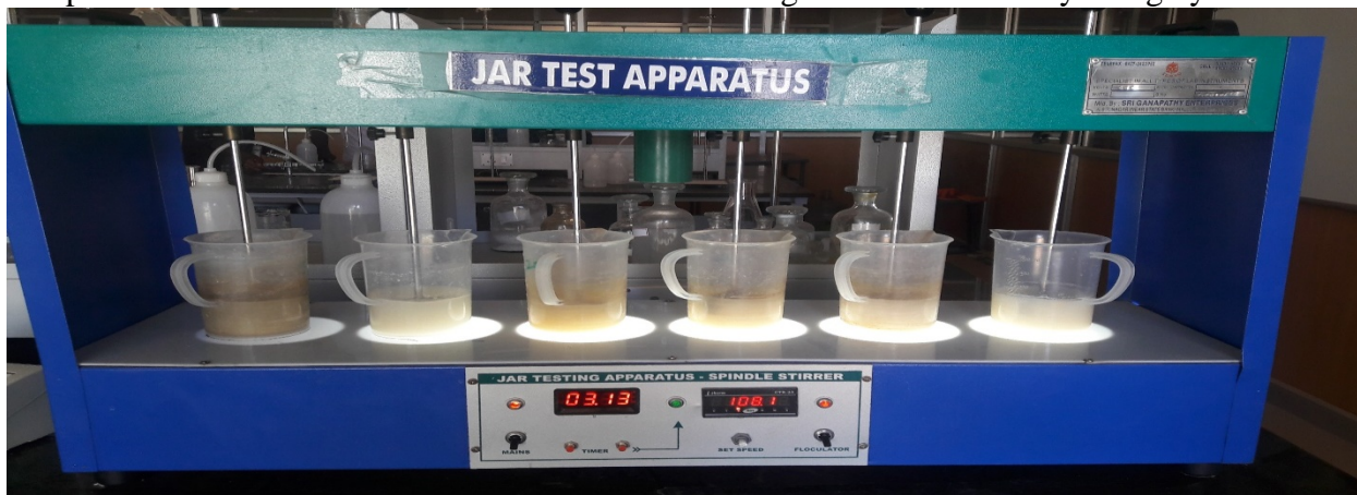
Fig 5.1 Jar test of moringa olifera seed
