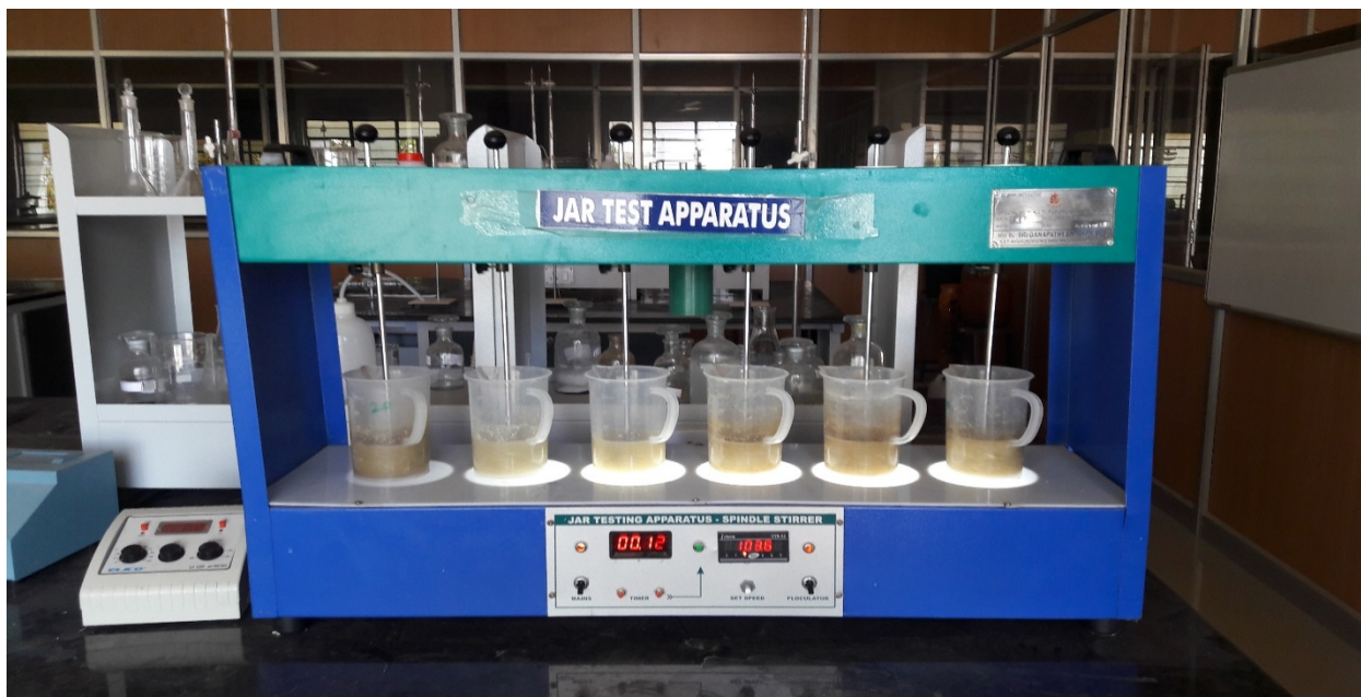
Fig 5.3 Jar test of jackfruit labab
