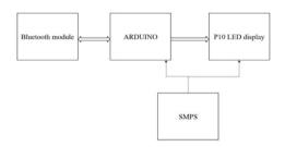
As we seen in the above figure there are 2 interfaces between bluetooth module and arduino and between arduino and display. The complexity of coding substantially increases, but once programmed the module works at its robust best since it is a embedded system and not a general purpose computer. The design procedure involves identifying and assembling all the required hardware and ensuring fail safe interfacing between all the components.
