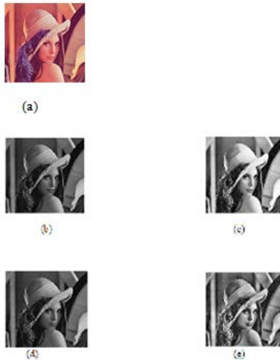
Figure 3.1 Lena.jpg (a) colour image (b) grey scale image (c) histogram equalization image (d) Imadjust image (e) CLAHE image
