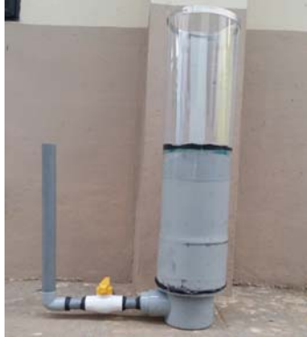
Fig.5 Apparatus for measuring permeability of pervious concrete by falling head permeability
