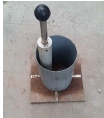
Fig.1 Cylindrical measure and standard proctor hammer as per ASTM C 1688
