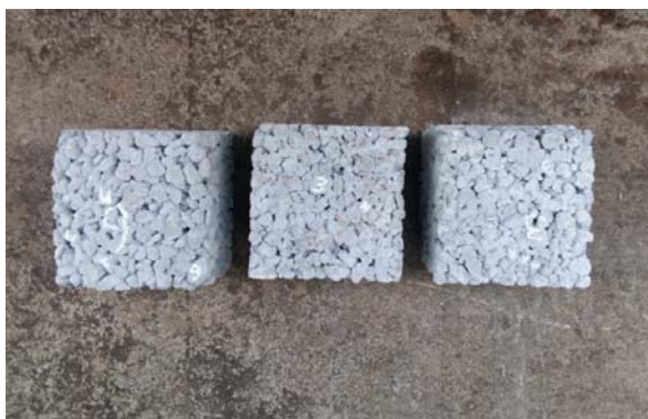
Fig.2 Cube specimen for conducting compression test
