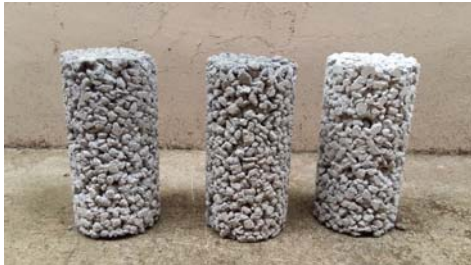
Fig.4 Cylindrical specimens for conducting falling head permeability test
