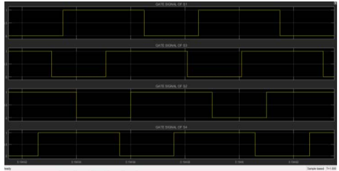
Fig.12 Waveform of Gating signal for MOSFETS: This figure shows the gate signal of the inverter at the primary side with the different states of operation i.e active state, shoot through state, and zero state.
