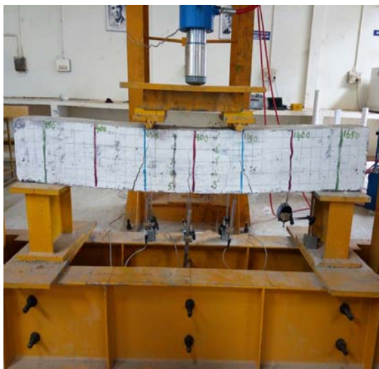
Figure 18 Ultimate Load Deflection Profile
