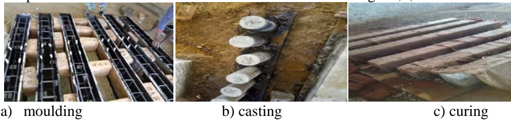
Figure 2 moulding, Casting and Curing of Specimens
