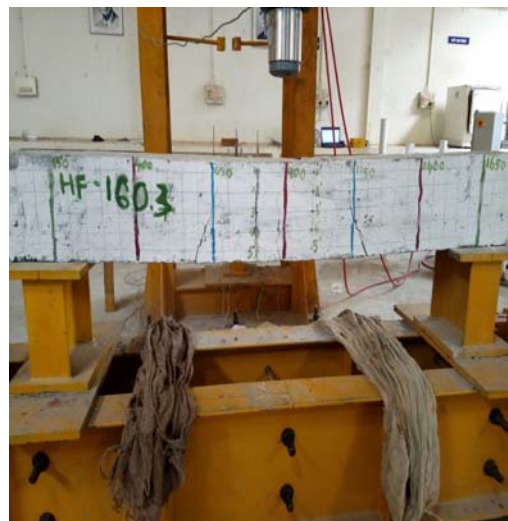
Figure 19 After load removal beam regain its normal position
