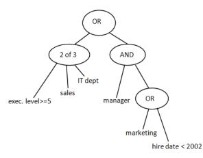
Figure 4: Access Tree with OR and AND gates
