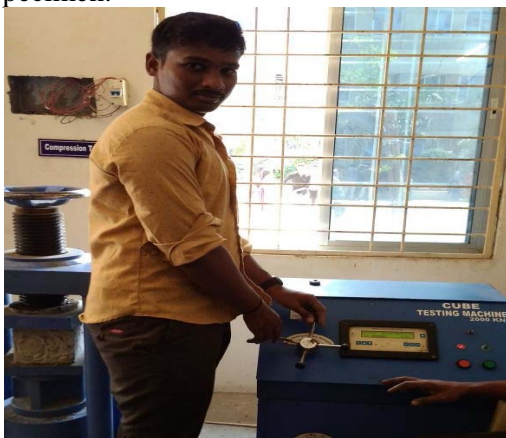
Fig.3.3 compressive strength of cubes
