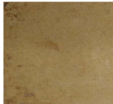
Fig. 8. A sample composites plate (weight fraction of citrus limetta particulate - 30%)
