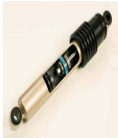
Figure1.1 Acceleration Sensitive Damping type shock absorber
