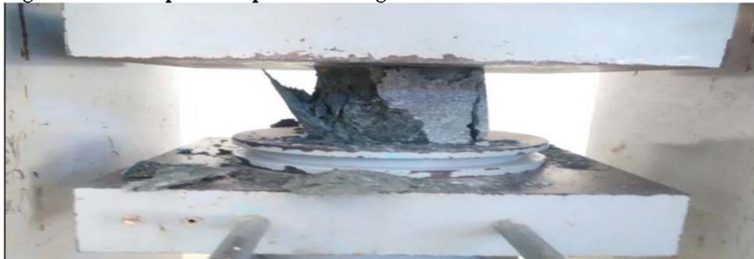
Figure 3 Test setup for compressive strength
