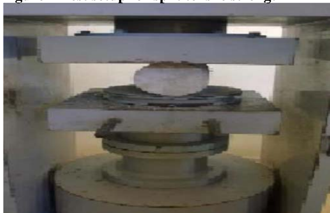
Figure 4 Test setup for split tensile strength
