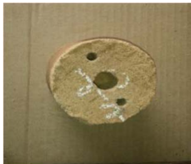
Figure 4: CO 2 – Silicate Mould after drilling
