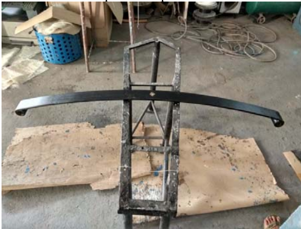
Fig(3.3.1(a)): Leaf spring arrangement
