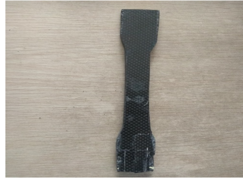
Fig 4.2 (c): Specimen after Tensile test
