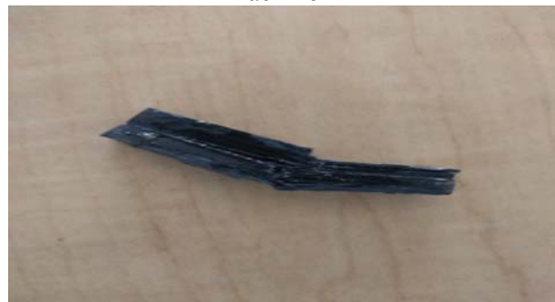
Fig(4.5.3 (c)): Specimen after Charpy test
