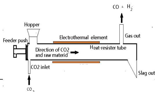
Fig. 6. push-rod type electric gas generator view diagram
