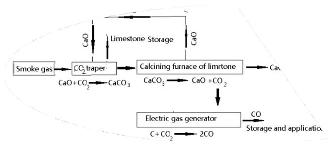
Fig. 5. Cyclic reactions between gas production and  $CO_2$  capture by  $CaO$
