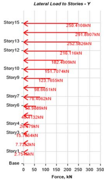
Figure 6 Load acting due to eq y
