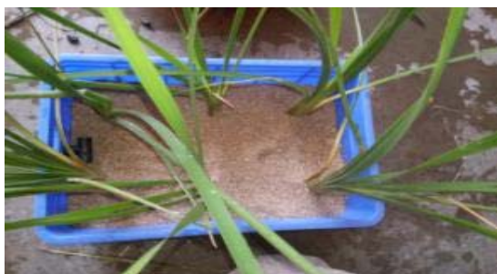
Photo 3: Filling of graded soil layers to supply of Sullage
