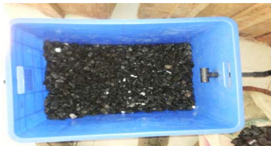
Photo 1: The middle part of the tank was 10-20mm pebbles and above it coarse sand.
