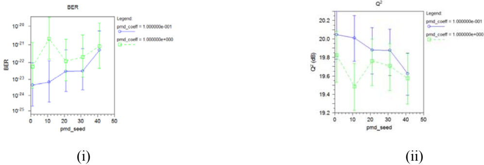
Fig. 3(a) pmd_seed v/s BER and pmd_seed v/s Q^2 dB response of RZ modulation format for \lambda_8
