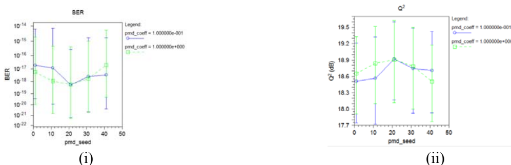
Fig. 3(b) pmd_seed v/s BER and pmd_seed v/s Q^2 dB response of NRZ modulation format for \lambda_8
