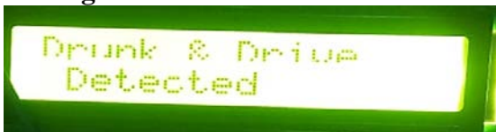
Fig.8:LCD Display when Alcohol consumes
