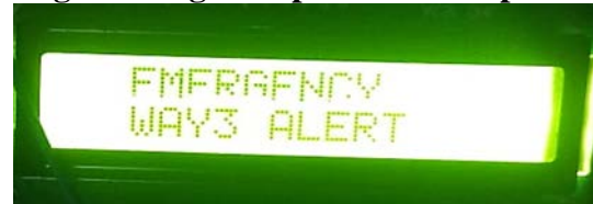
Fig.12:LCD Display when Emergency Occurs
