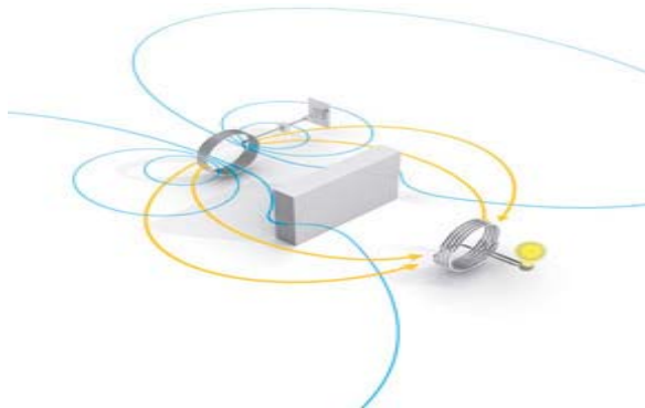
Figure 5: Two idealized resonant magnetic coils
