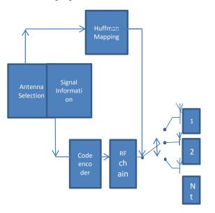
Figure 1: RF chain model with Huffman Coding
