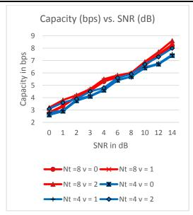
Fig 4: Channel capacity values for Nt=4 and 8 for different **v values**
