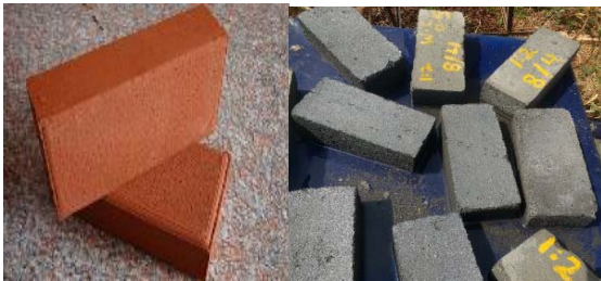
Fig. 1 – CLC bricks V/S clay bricks (ordinary bricks)
