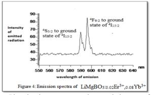
Photoluminescence characteristics of LiMgBO<sub>3</sub>: $_{0.02}$ Er<sup>3+</sup>, $_{0.08}$ Yb<sup>3+</sup> is shown in **figure(4**). It shows two upconversion emission peaks at 590 nm and 596 nm when excited in infrared region. It is due to mixed transitions from <sup>4</sup>F<sub>9/2</sub> and <sup>4</sup>S<sub>3/2</sub> to <sup>4</sup>I<sub>15/2</sub> in the Er<sup>3+</sup>.
