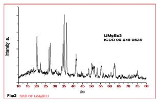
**Fig.2** shows the powder X-ray diffraction (XRD) patterns of LiMgBO<sub>3</sub>: $_{0.02}$ Er<sup>3+</sup>, $_{0.08}$ Yb<sup>3+</sup>, and it was found to be in good agreement with the reported standard data in ICDD file no. 00-049-0528. The result clearly implies that the obtained samples are single phase and the doping of Er<sup>3+</sup> and Yb<sup>3+</sup> does not cause any significant change to the detection limit of the technique in the host structure.
