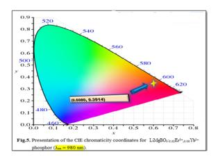
CIE chromaticity coordinates for LiMgBO<sub>3:0.02</sub>Er<sup>3+</sup>,<sub>0.08</sub>Yb<sup>3+</sup> phosphor at  $\lambda_{ex} =$  980 nm for emission wavelength 596nm are shown in the figure (5). It shows the colour of emitted light was orange.
