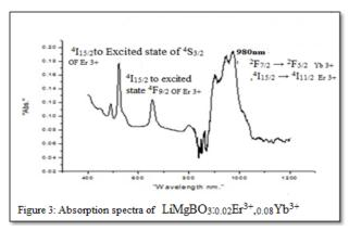
To decide excitation wavelength of sample for study of UC we did the absorption study of sample using Shimadzu UV-VIS-NIR Spectrophotometer in the range 400 nm to 1200 nm. Figure(3) shows absorption spectra of LiMgBO<sub>3</sub>: $_{0.02}$ Er<sup>3+</sup>, $_{0.08}$ Yb<sup>3+</sup>.
