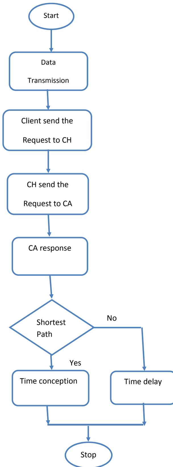
The above diagram gives the data-flow of the proposed system, initially all the nodes will be initialized and source will start the data transmission process, cluster head will initiate the request process to the CA and then CA will respond to the request, then a shortest path is evaluated and data is transmitted to the destination.
