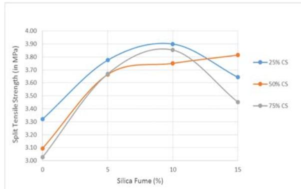
Figure 3 showing the comparison of Split Tensile strength with various percentages of Copper Slag and Silica Fume at 28 day's age of concrete
