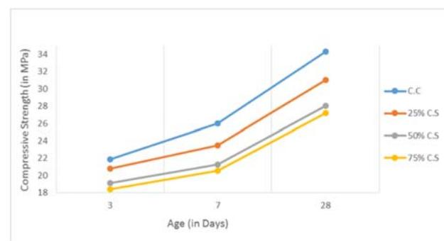
Fig No.1 Variation of cube compressive strength with the controlled concrete by replacing copper slag at 25%, 50% and 75% with sand
