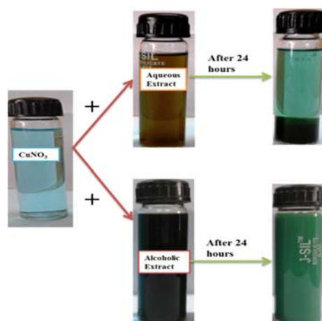
Fig.1 The change observed in the color of the solutions with the progress of the reduction of \text{Cu}^+ ions by the (a) aqueous extract and (b) alcoholic extract of Swertia chirayita with time.
