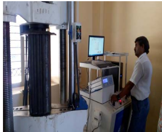
Fig 4. Innovative HSS column setup and equipments
