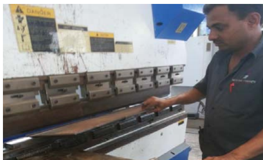
Fig 2. Cold forming of initially flat plates into corrugated steel plates using press brake machine.
