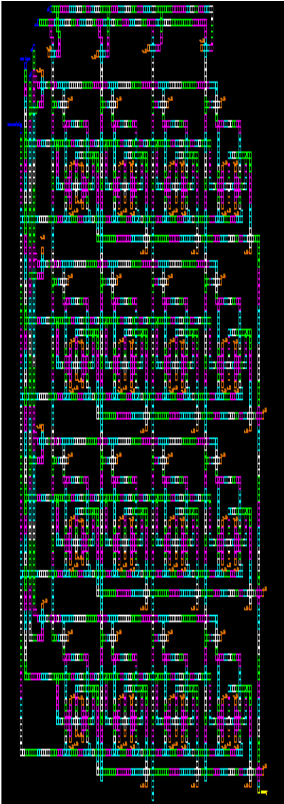
Fig. 10 -16 bit RAM memory implementation using proposed & modified memory cell
