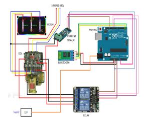
The bluetooth module is connected to arduino ATMega328 microcontroller, digital pin no 1 is used for sending (TX pin) and digital pin no 0 for receiving (RX pin) and here bluetooth module is powered with onboard 5 volt power supply but HC-05 module power ranges from 3.3v to 5v(VCC pin) and GND pin as ground. The Relay module used here is 2 channel PNP type that is
