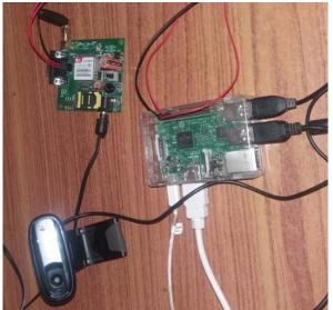
Fig 3 Interfacing of USB camera and GPRS module to Raspberry Pi
