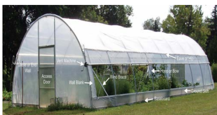
Fig 7: Common high tunnel terminology
