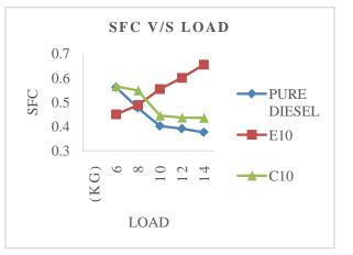
The diesel blend of ethanol diesel blend fuel specific fuel consumption (SFC) is pretty higher than cotton seed oil and diesel. The ethanol diesel blended fuel (E10) SFC is also higher than the diesel among the entire blend. But the diesel blended of cotton seed oil (C10) is closer to diesel. The all blended fuel at a far cry from segment, the specific fuel consumption is gently decreasing along with increasing load in cotton seed oil and diesel.
