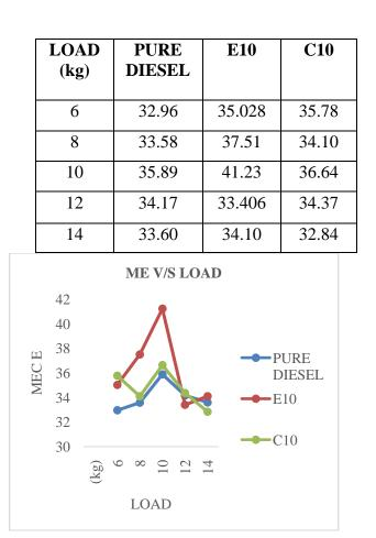
The cotton seed oil (C10) ME is also higher than the diesel but lower than the E10, among the entire blend. The all blended fuel at a far cry from segment, the mechanical efficiency is gently increasing along with load from 6kg to 10 kg after than slowly decreasing.
