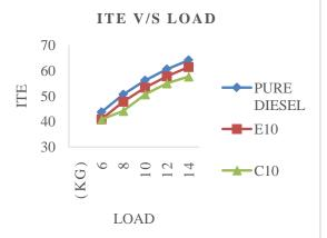
Ethanol blended fuel (E10) is closer to diesel and higher than the cotton seed oil, among the entire blend. The all blended fuel at a far cry from segment, the indicated thermal efficiency is gently increasing along with the pretty increasing load.
