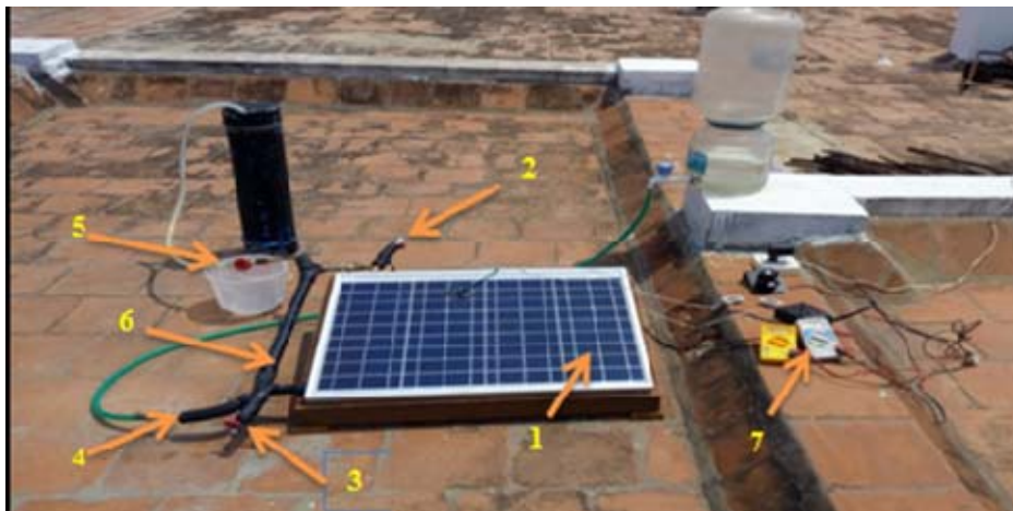
Fig 4. Experimental setup of PV/T systems with counter flow heat exchanger: (1) PV/T system, (2) nanofluid inlet, (3) nanofluid outlet, (4) water in, (5) hot water out, (6) counter flow heat exchanger and (7) instruments.
