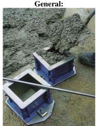
In order to achieve the objective of the present study, an experiment program was planned to investigate the effect of the sugarcane baggase ash on properties of cement replaced by sugarecane baggase ash in different percentage i.e. 0%, 5%,10%,15%respectively.The various parameters are investigated and test are performed such as compressive strength.
