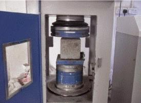
The test was conducted according to IS CODE 516-1959<sup>11</sup>. Specimens were taken out from curing tank at the age of 7, 14, and 28 days of moist curing and tested immediately after removal from water. Surface water was allowed to drip down. Specimens were tested on 200 TONES CAPACITY OF UNIVERSAL TESTING MACHINE UTM . THE POSITION OF THE CUBE WHILE TESTING WAS at reight angles to that of casting position .
