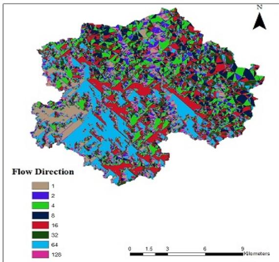
**Fig.8:** Flow Direction grid
