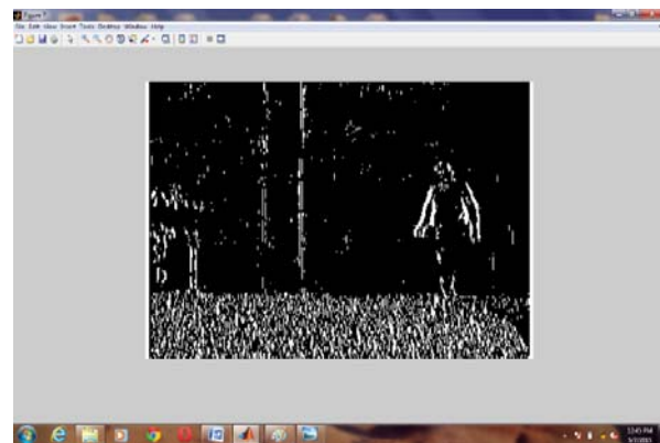
Figure 6.7: Frame processing for edge detection
