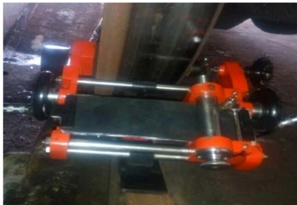
Fig . 6.1. wheel profile gauge
