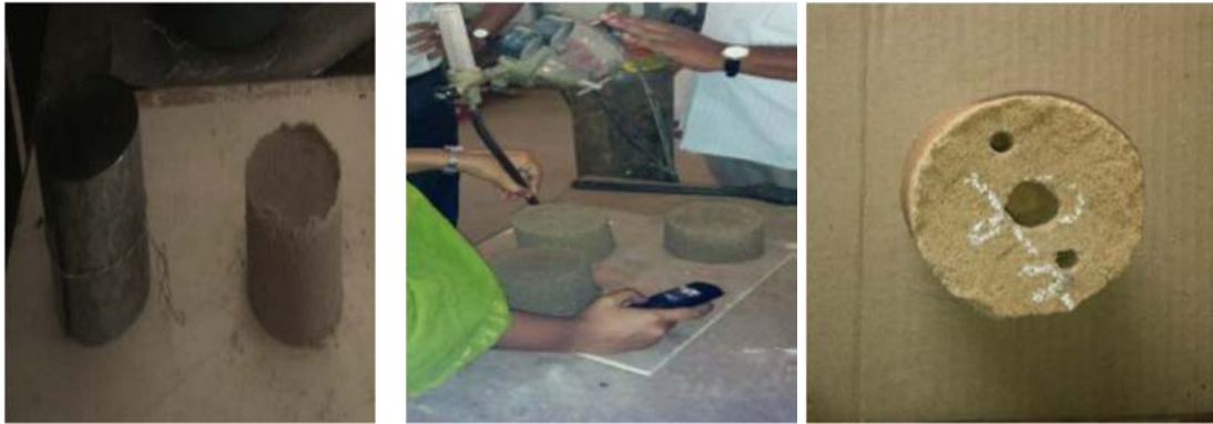
Figure 2; Mould Cavity of Sheet Figure 3: Passing of CO 2 gas Figure 4: CO 2 – Silicate Mould after drilling process metal with co2 silicate moulds.
